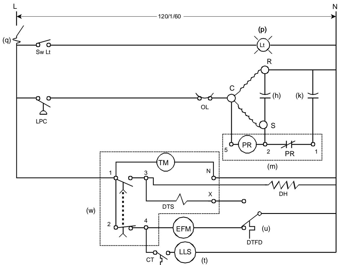
117. Identify the two (2) over-current devices in the schematic.
